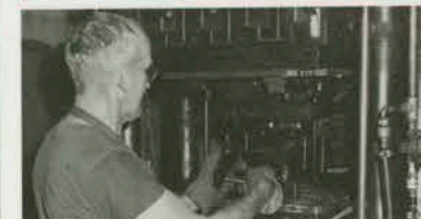
Compression molding machines showing the die which forms a preheated pellet into a clipper case.
