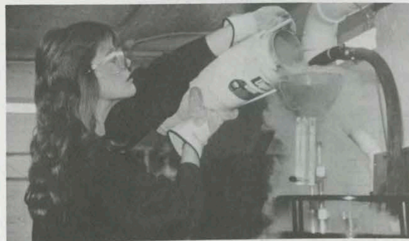
At Yerkes Observatory, liquid nitrogen is poured into an instrument which will be used to detect infrared radiation.
