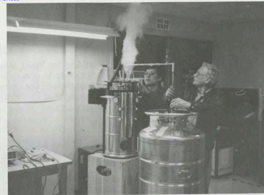
KAO and Yerkes Observatory staff pump liquid helium into an infrared detector system shortly before it is carried aloft on telescope aboard the Kuiper Airborne Observatory.
