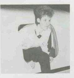
Should it become necessary to leave the aircraft in an emergency, all available exits should be used. The Piper Cheyennes and the Diamond Jet all have an emergency exit over the right wing which is also the window for the passenger seated in the forward (aft facing) club seat on the right hand side of the airplane. To operate the exit,
