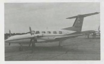
The Piper Cheyenne III, (N620MW) is easily identified by it's high "T" tail. It seats eight passengers plus one pilot, and can be recognized from the inside by it's lighter beige interior and the fact that the last two passengers sit side by side on a "bench" seat when eight passengers are carried. It cruises a little faster than the other Cheyennes (260 knots true airspeed) and makes the trip between Minneapolis and Warroad 5 to 10 minutes faster.
