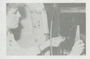
oxygen is included in this pamphlet. Please read it carefully. Normally the pilot will open and close the main cabin door. In an emergency a passenger may need to open the door, and if able, assist other passengers in exiting quickly. To open the main door in all three Cheyennes, pull on the small silver knob (located to the left of the large handle) and rotate the handle counter-clockwise.
